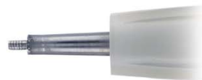
Worn screw thread with brand X tips
